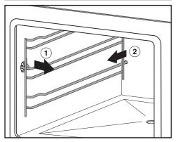
■ Pull the side runners out first at the side ①, then at the back ② of the steam oven
